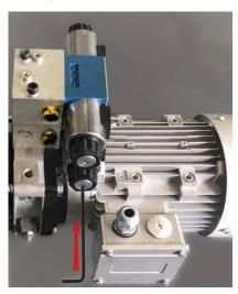
With the end of the Allen key, press the distributor's brass coloured nozzle and, at the same time, pull the wheelstop's reinforcement leg to make the wheelstop enter. The reinforcement leg must not be pressured on the truck's wheel. If the wheek-stop does not re-enter at all, do the same operation with the opposite coil.
