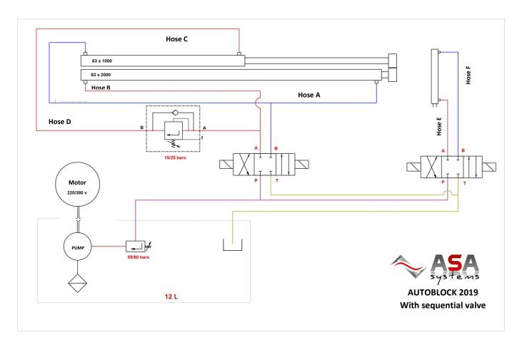
The hydraulic part includes a hydraulic unit tared to 60 bars.
