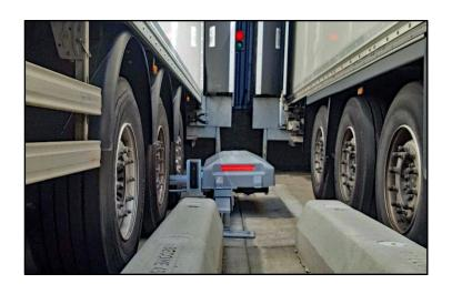
Autoblock is a machine designed to secure docking procedures and merchandise transhipment by immobilizing the truck's trailer while the loading / unloading procedure takes place.
