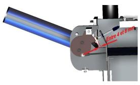
Connect by screwing the connector(s) on the female plugs under the control unit.
