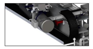
Note: The hydraulic unit must be moved (2 screws under the block) to be able to remove the rear axle.
